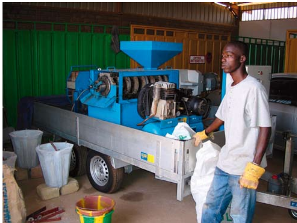
A Mali Biocarburant employee beside the moveable press used to produce oil from jatropha nuts Photo: Bart de Steenhuijsen Piters
