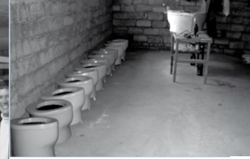
Cement urine diverting toilet seats as produced by WECF partners for the sanitation improvement programme
