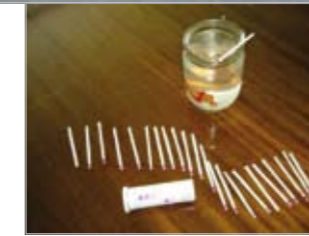
Figure 5: Nitrate test strips are cheap tools to give a reliable and fast estimation of the nitrate concentrations in drinking water
