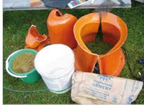
Figure 50: The urine diverting toilet seat is almost finished
