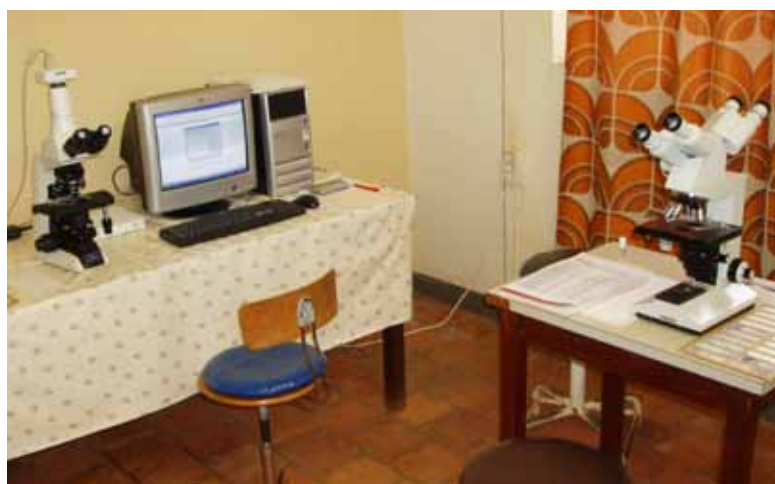
The camera connected to the left microscope is used to digitise tissue samples and send them to specialists.
