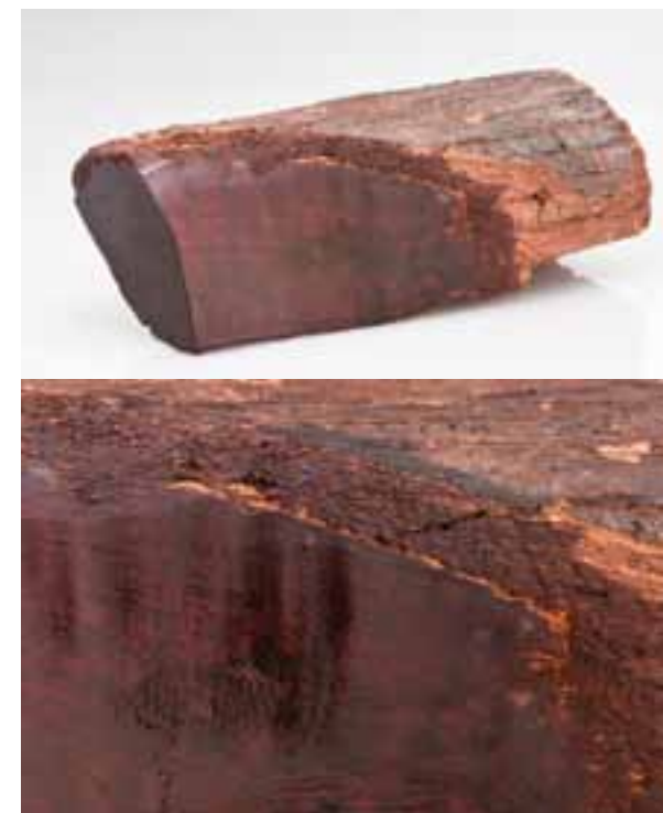
Photo 2.1. Sometimes a keen observer sees an apparently rotten stem on the forest floor, lying there for perhaps half a century or more, which upon inspection proves to be a piece of core-wood of Letterwood, hidden in a mantle of decayed sapwood. Letterwood Brosimum guianense , Moraceae, is a very durable, dense and heavy wood. Local varieties show an attractive pattern of blots. It was one of the first export products of Suriname and it was gathered by hand. (Photo J.Franco)
