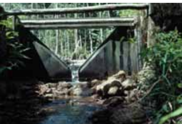
Photo 6.2. Weir to measure water flow, Kabo, 1982. (Photo K.E. Neering)
