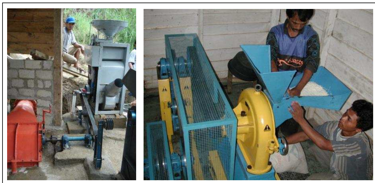
Productive Use of MHP by mechanically direct driven milling machines in Sulawesi and Java.
