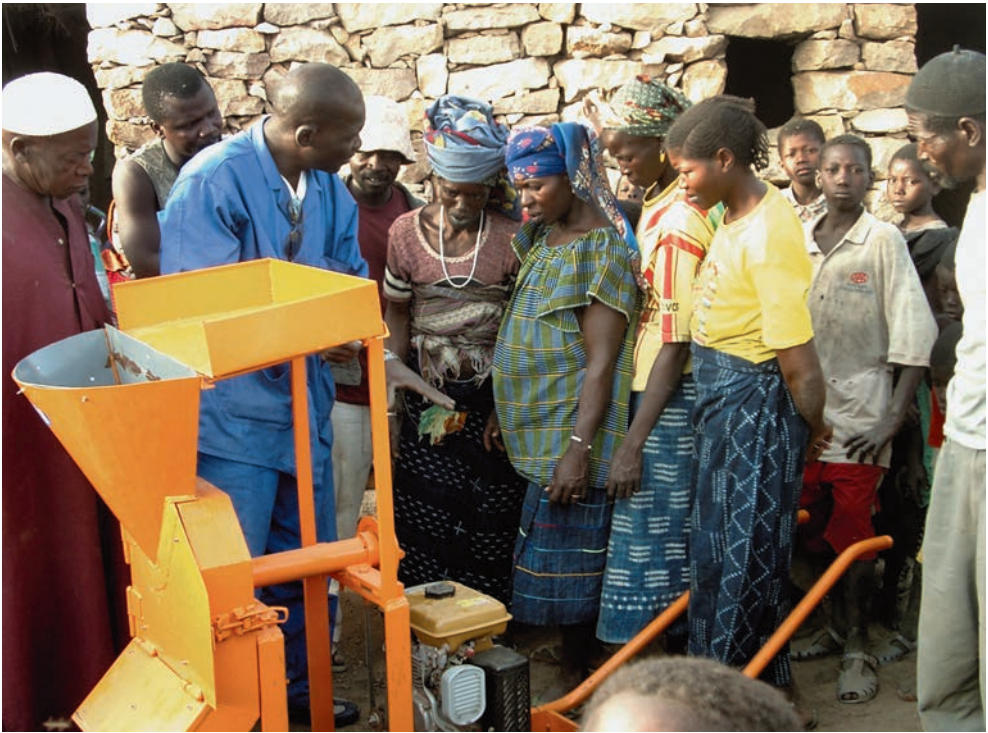
Testing introduction of improved slicers for the production of dried shallot chips
