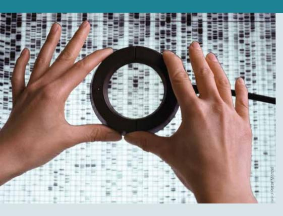
The heart of the matter: circular computer scanner used to read sections of DNA sequencing autoradioarams
