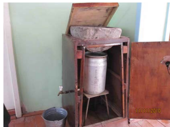
Photo: Marmora filter for the treatment of river water
