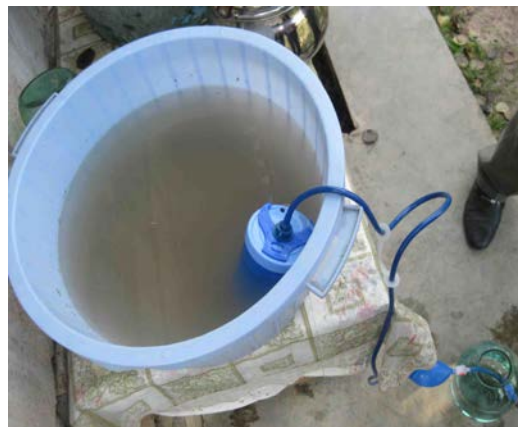
Photo: Testing the tulip filter in a common household, using a common water source
