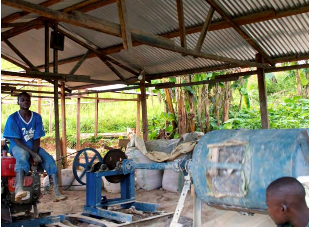
Photo 7: mechanized crushing of the large stones in Mongbwalu (Djugu)
