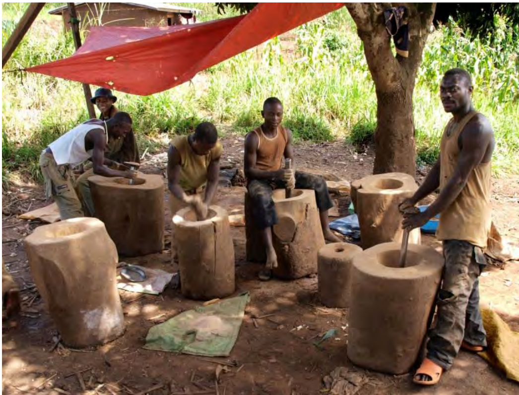
Photo 8: crushing of the small stones in Balanzana (Irumu)
