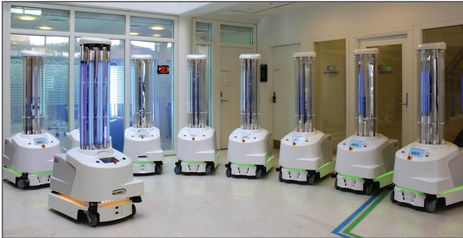
Figure 4. Disinfecting robot consisting of a mobile base equipped with multiple LIDAR sensors and an array of UV lamps mounted on top. Credit: UVD Robot, see: “Hundreds of These Ultraviolet Disinfection Robots Are Being Shipped to China to Help Fight the Coronavirus Outbreak”, online e-picture, under “Autonomous Robots Are Helping Kill Coronavirus in Hospitals”, IEEE Spectrum , 11 March 2020, https://spectrum.ieee.org/autonomous-robots-are-helping-kill-coronavirus-in-hospitals .
